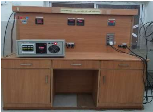
Testing Arrangement for RCB/ECB
